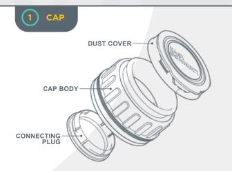
The easyconnect cap is resealable and leak-proof. The connecting plug safely contains the remaining product until the next usage.
