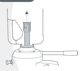
To empty the container, the coupler probe pushes the internal connecting plug of the easyconnect cap into the container, thereby allowing the liquid contents to be emptied via the coupler into the tank.
