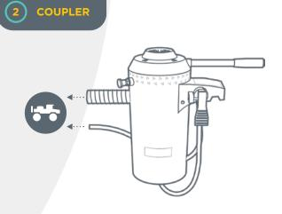
The coupler connects to a sprayer tank to transfer the product into the sprayer.
